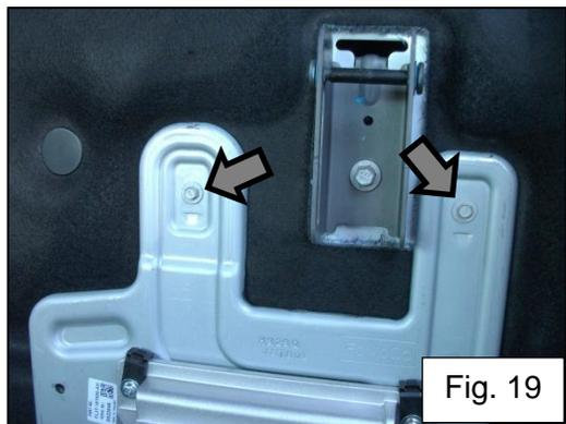
32. Remove the passenger side factory subwoofer mounting stud. Fig. 20
